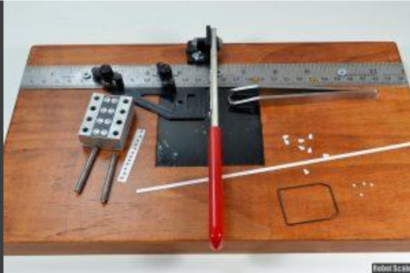
21 - Making supports/punching circles
